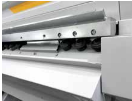
Easily accessible forming rolls for maintenance work.
