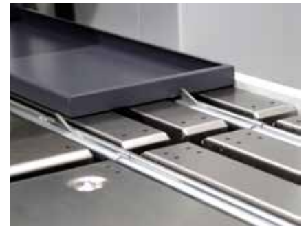
Part lined up with the squaring arm.
