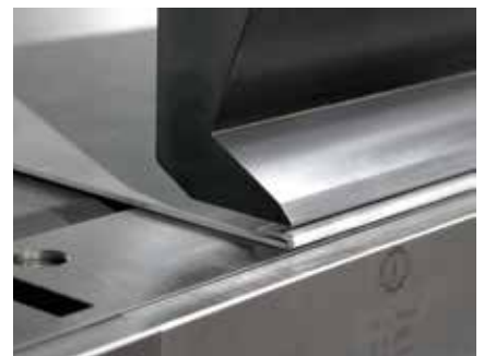
At the same time, the PowerBooster offers impressive performance when hems need to be closed.
