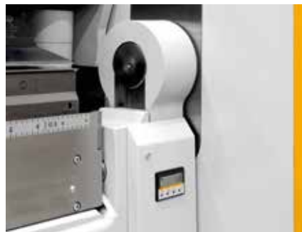
Optional digital display for folding beam adjustment.
