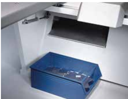
Small parts chute for sorting small blanks.
