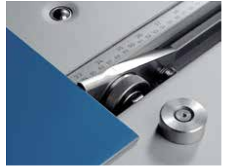
Front stops (available also with a precision scale) allow an accurate part positioning.
