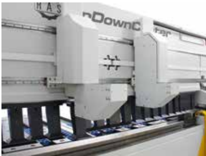
The automatic tool changer (78.33-2 & 78.43-2) sets up of even heavy tools.
