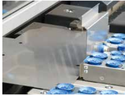
High flexibility in handling due to front suction cups and small part suction cups.
